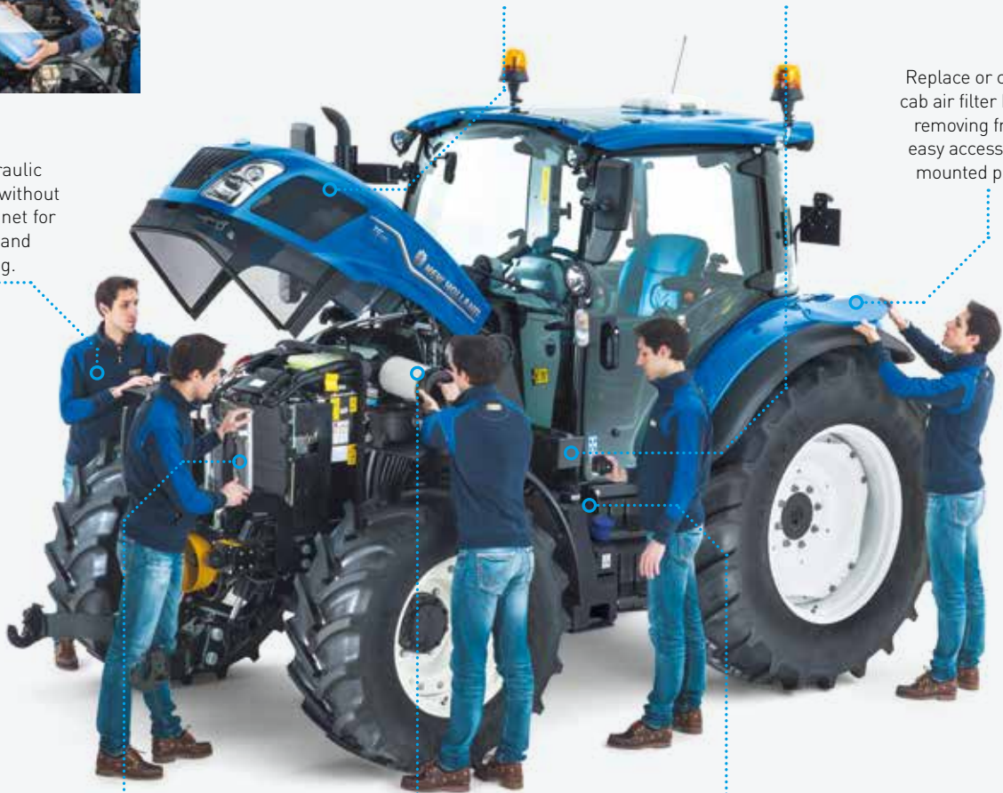
Single piece, lockable bonnet opens wide for full servicing access.
