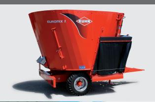
The single auger EUROMIX I comes in 8, 10 and 12 m³ versions with a vertical auger, providing mixed rations for all types of livestock farms. The shape of the tub and the auger design were specially engineered to ensure optimum circulation of the forage products in the machine and guarantee an even mix. The counter-knives are articulated at the top to provide a large chopping surface.
