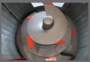
All the auger parts (coils and cones) are made of K-NOX to protect the entire unit. The auger is more resistant to abrasive fodder and acidic silage juices.
