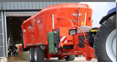
Available in 28, 33, 39 and 45 m<sup>3</sup> versions, the triple vertical auger EUROMIX industrial range features extra-large dimensions. The 28 m<sup>3</sup> models feature an overall height starting at 2.74 m and can manoeuvre through lower buildings.
