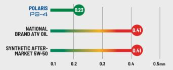
ASTM D4172. In 3rd party testing against 9 competitive products Polaris had 40% or better wear protection compared to all of the tested products. Numbers represent mm of wear scarring measured. Test measures wear at contact points, wear scar is measured for its length and wild (In units of mm). Lower wear numbers mean better wear protection and friction reduction.
