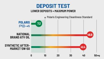
ASTM D6335. In 3rd party testing against 9 competitive products Polaris PS-4 had less than half the deposits compared to the next closest product. No other tested products met Polaris Engineering standards for deposit cleanliness. Test measures mass of deposits in mig in high term, high stress test cycles. Higher deposits will impact engine power and performance.
