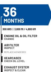
INSPECT FOR LEAKAGE OR CARBON BUILD UP AT JOINTS INSPECT & CLEAN SCREEN TYPE SPARK ARRESTOR
