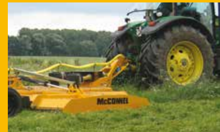
Above: High hitch configuration Right: Low hitch configuration with optional Scharmuller ball hitch
