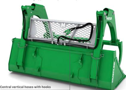
Hoses are kept out of harm's way on the loader carrier frame, preventing damage during hookup. Hose-holding hooks are also available for storage when not in use.
